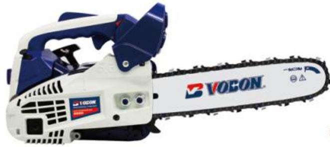
Model: 2500 GASOLINE CHAIN SAW Displacement 25.4cc Engine 2 Stroke Engine Guide Bar Size 10"/12" Idling Speed 3000 rpm Rated Power Input 0.9 KW
