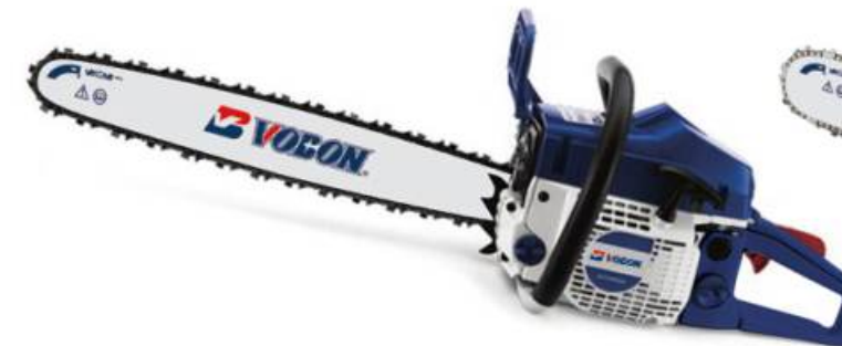
Model: 5200/5800 GASOLINE CHAIN SAW Displacement 52/58cc Engine 2 Stroke Engine Guide Bar Size 16"/18"/20"/22" Idling Speed 3000 rpm Rated Power Input 2.2/2.4 KW
